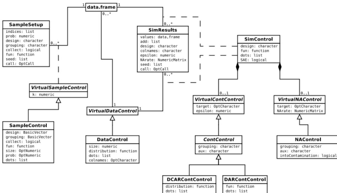
Figure: Simplified UML class diagram of simFrame
