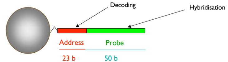
Each silica bead is 3 microns in diameter
